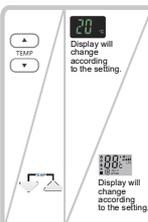
Press TEMP/TIMER ▲ or ▼ to set the display temperature. The temperature can be set between 16°C and 30°C. Recommended temperature: 26°C-28°C
