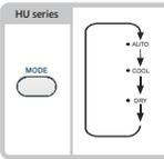
Press MODE to select the desired operation. (The indicator will light up and a "beep" sound will indicate changing setting)
